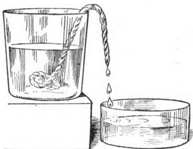
FIG. 43. — An Example of Capillarity.
